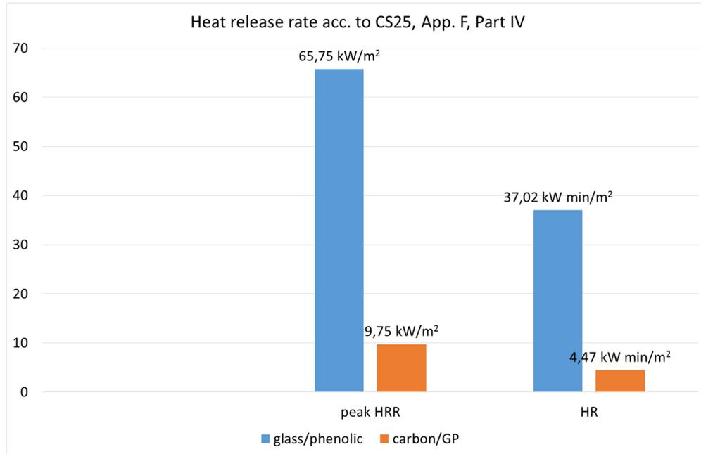
**Figure 6 - Comparison of Heat Release Rate and Heat Release values of carbon/geopolymer composite with referential glass/phenol**
