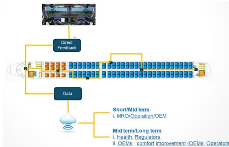
**Figure 11 - IFCAS concept architecture (cabin/cockpit pictures Embraer)**
