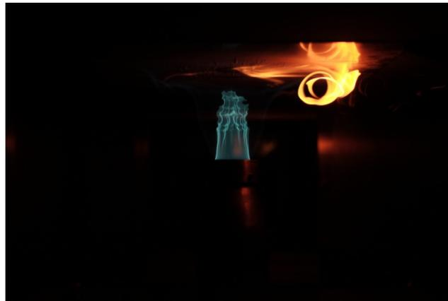
**Figure 4 - Internal damage induced by impact affecting the gas release and ignition on the material surface**
