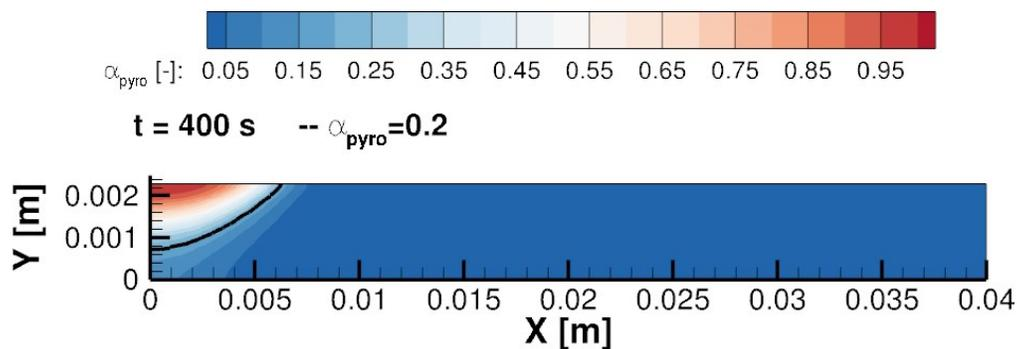
**Figure 5 - Final pyrolysis evolution function field of the T700GC/M21 ISO simulation exposed to a 101.2 kW/m<sup>2</sup> laser beam (ONERA MoDeThec Solver)**
