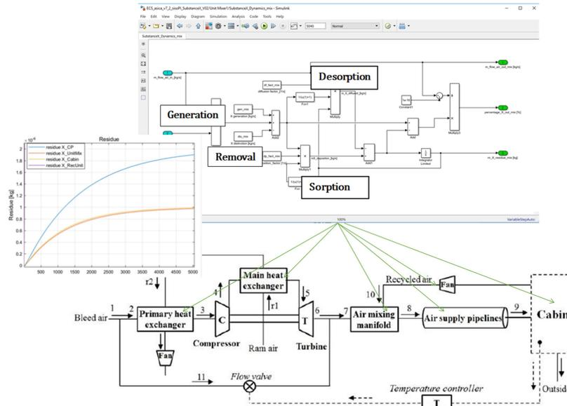
**Figure 10 - Cabin air quality building block for aircraft environmental control system (ECS) model with ECS schematic from literature<sup>1</sup>. Verification of the integration of the building block**
