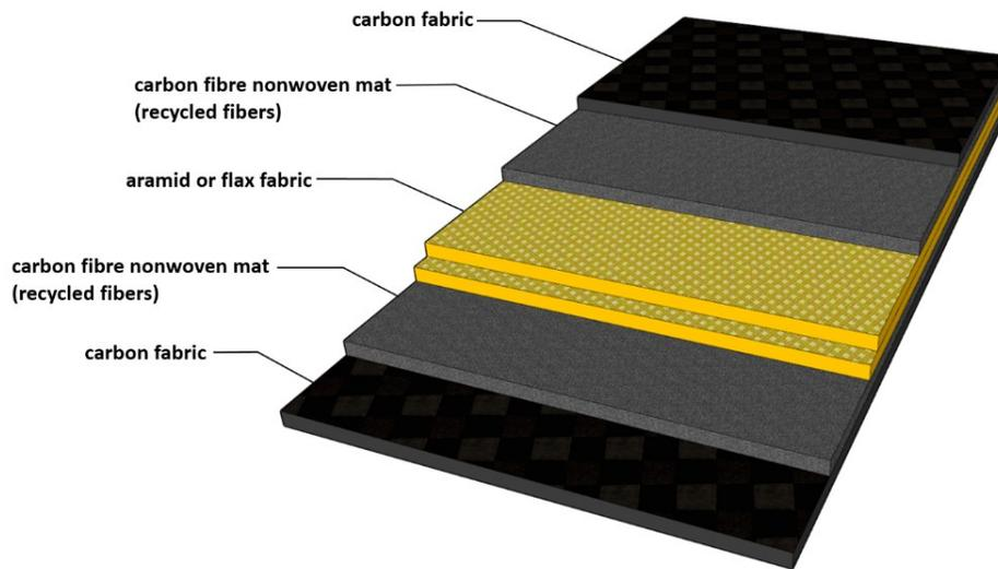
**Figure 8 - Lay-up of the geopolymer test panel containing layers of recycled and ductile (natural) fibers**
