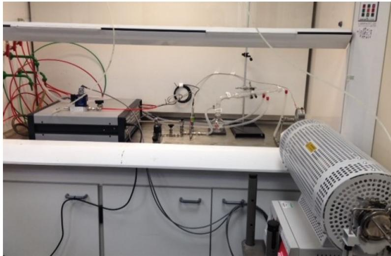
**Figure 9 - Experimental apparatus for characterisation of gas emissions at elevated temperatures in realtime using commercial gas sensors and thermal desorption tubes**
