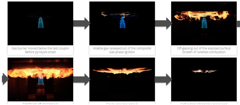
**Figure 3 – Overview of the successive events occurring during the fire exposure onto the composite test coupon with the FIRE facility**
