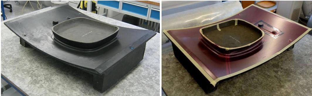
**Figure 13: The raw (left) and protected by aDiatex A5000 release film (right) mold of the first demonstrator**
