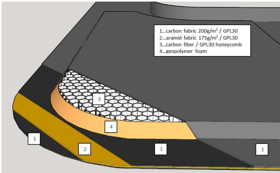
**Figure 14: Lay-up scheme of the structural demonstrator (molding A)**
