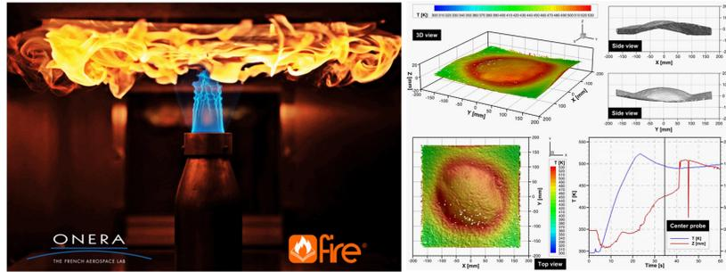
**Figure 2 - 3D reconstruction of temperature measurements on the back surface of a composite laminate exposed to fire (FIRE facility @ONERA)**
