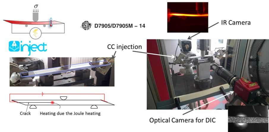
**Figure 1 - Injet facility used to study the influence of the high temperature on the fracture toughness of composite materials**
