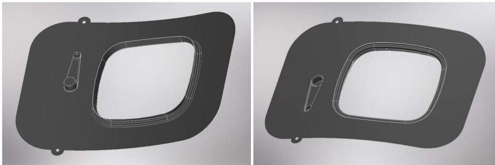
**Figure 12: Design of the first demonstrator – inner (left) and outer side (right)**
