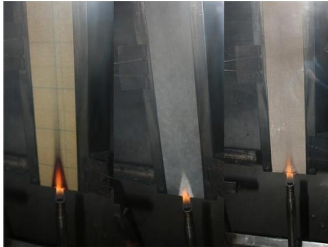
**Figure 7 - During the 12 sec vertical flammability test (glass fibre + phenolic resin reference (left), recycled carbon fibre + geopolymer (middle) and flax + geopolymer (right))**
