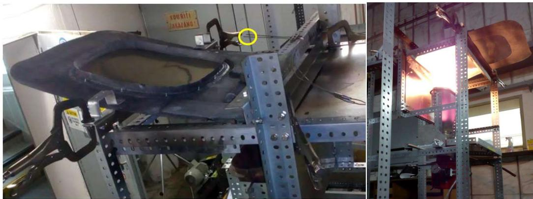
**Figure 16: Flame penetration test per CS 25, App. F, Part III - Two thermocouples (in yellow circle, see left) were set 100 mm above the back surface**
