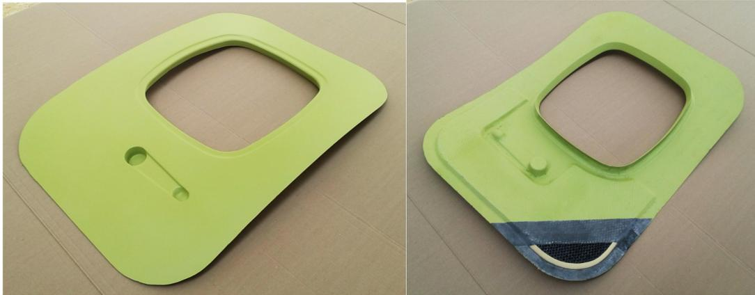
**Figure 15: Outer (left) and inner (right) side of the molding A (surface filled and painted)**
