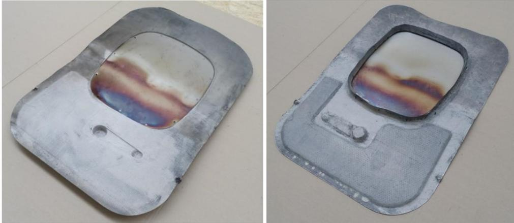
**Figure 17: Molding B after 10 minutes of the flame penetration test - Exposed side (left) and back side (right)**
