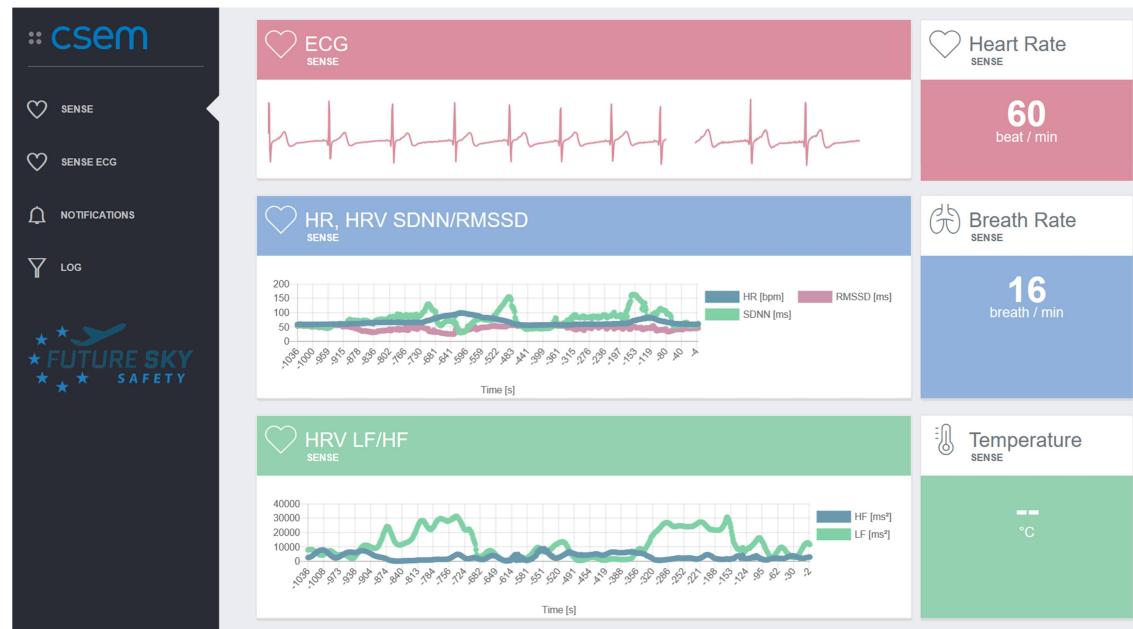
Figure 2: Visualization example of physiological signals from the smart vest via a simple web browser.
