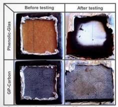
Specimens before and after test: GP shows almost no influence whereas phenolic resin is completely burnt off
