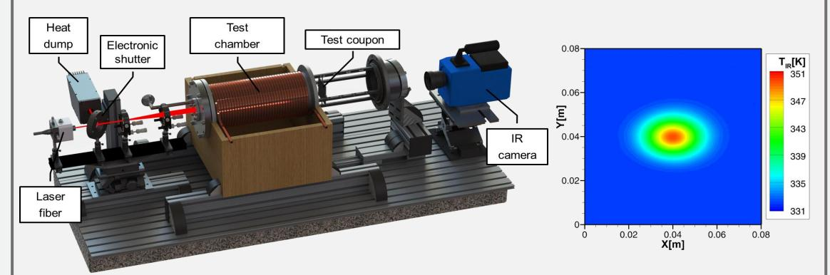
**BLADE facility developed at ONERA to characterise thermal properties** (thermal conductivity tensor and specific heat) of composite laminates
