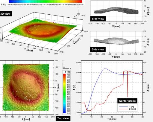
3D reconstruction of temperature measurements on the back surface of a composite laminate exposed to fire (FIRE facility @ONERA)
