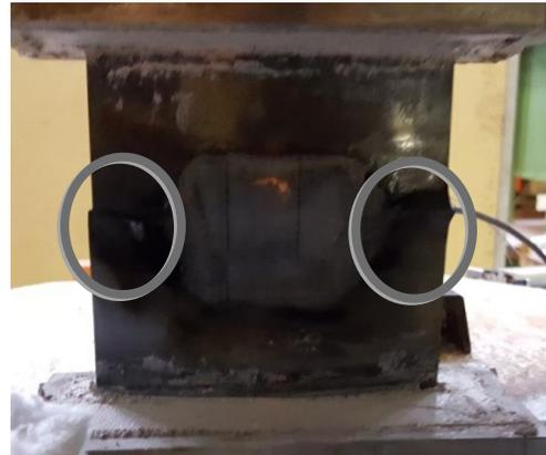
Specimen front after testing, stability failure visible at specimen edges
