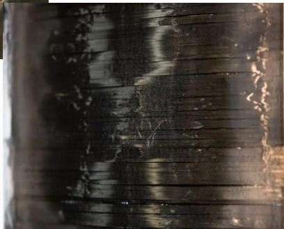
FML: No burn-through or decomposition on the inner side
