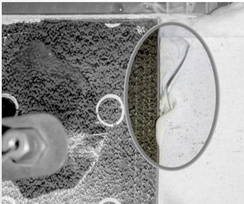
Delamination results in leakage of insulating gas
