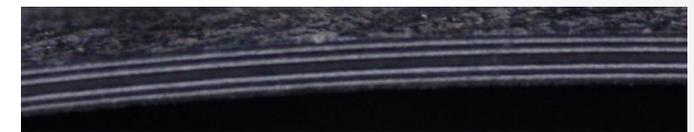
Manufactured FML cross section
