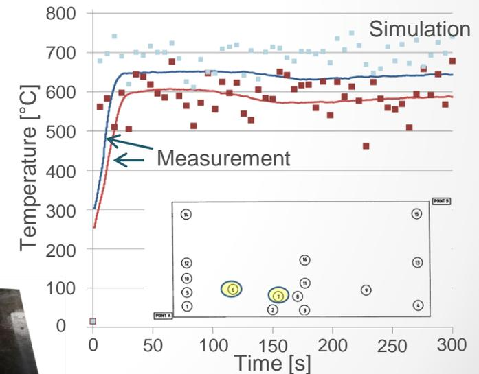
Comparison of temperature history between experiment (lines) and simulation (points) at 2 positions
