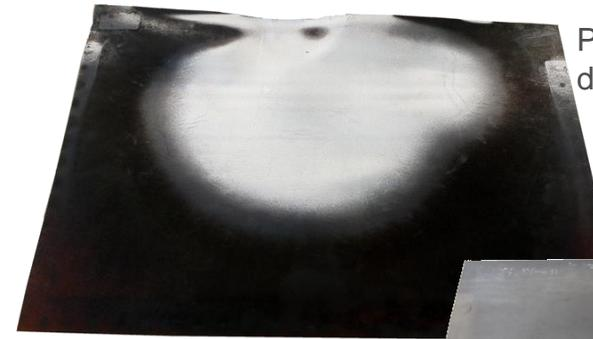
Phenolic-Glass: Completely decomposed matrix
