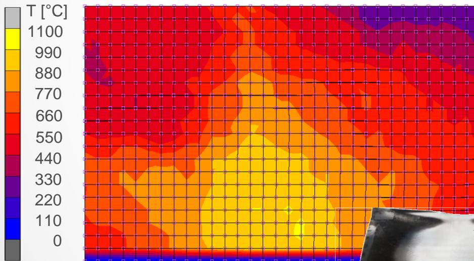
Comparison of temperature distribution of simulation to burnt area of a common phenolic-glas specimen after flame penetration test
