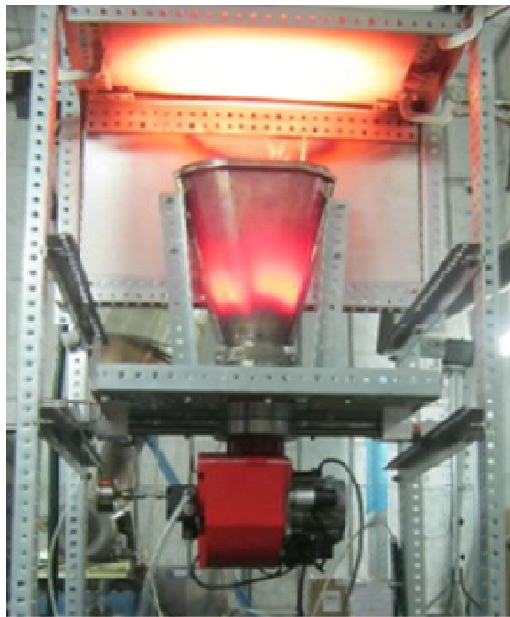
Figure 1: Flame penetration test - rig
