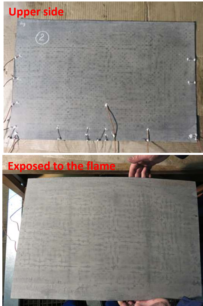
Figure 8: Specimen thermocouples installation
