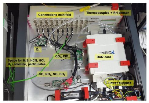
Figure 7 Sensors box equipped with COTS gas sensors. Labels are highlighted in yellow.
