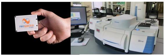
Figure 4 Miniature handheld FTIR vs. typical benchtop FTIR, taken from [89] and [90]
