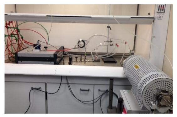
Figure 6 Experimental apparatus for characterisation of gas emissions at elevated temperatures in realtime using commercial gas sensors and thermal desorption tubes.
