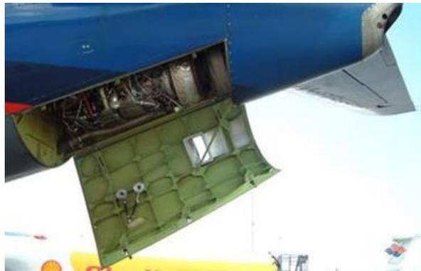
**Figure 4 Fire zone: Auxiliary Power Unit compartment**
