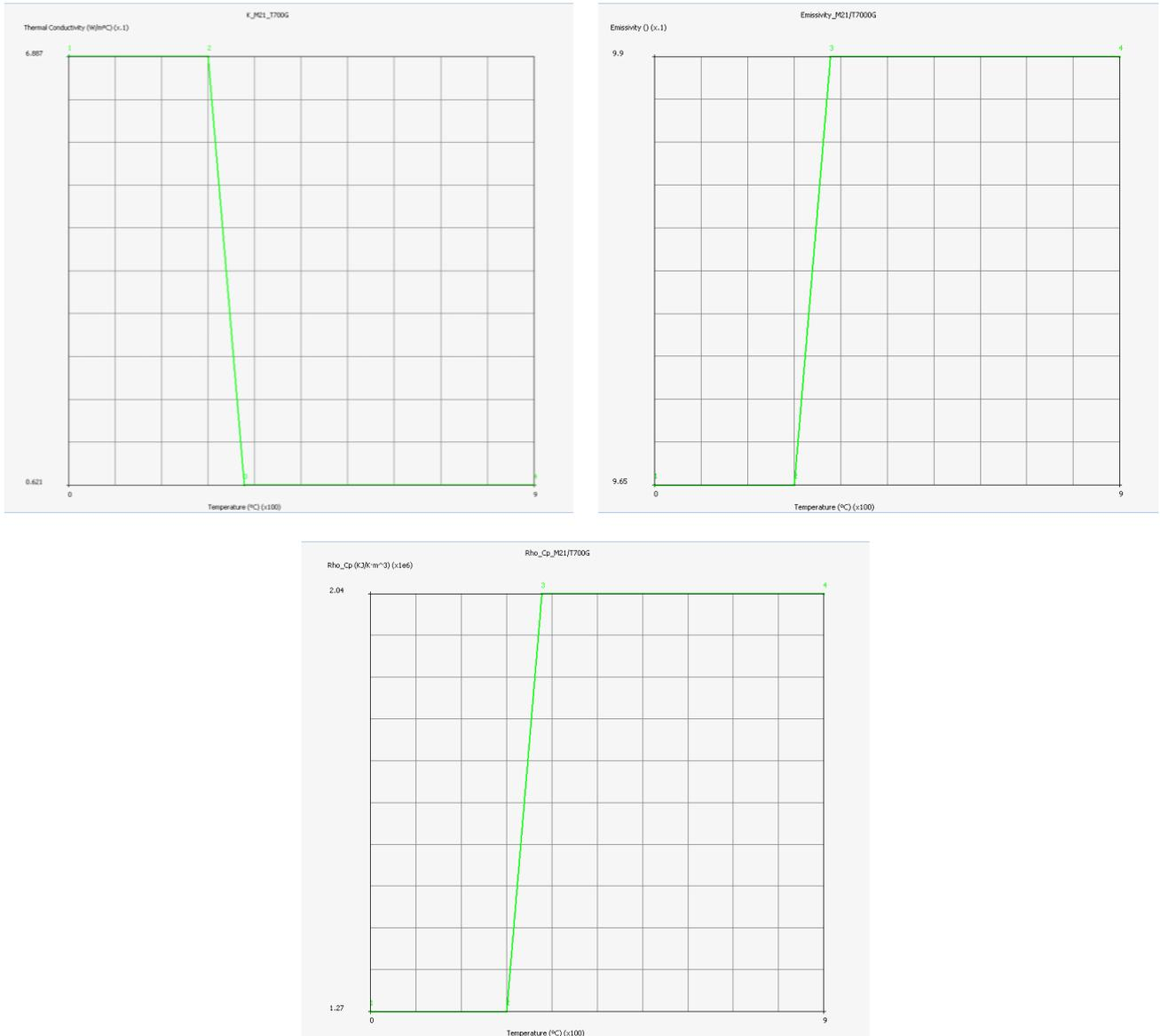
**Figure 85 M21/T700G thermal properties**
