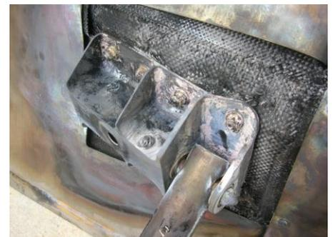
**Figure 3 Flame test on a hinge fitting**
