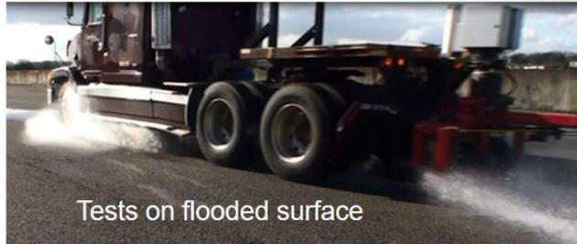
Tests on flooded surface
