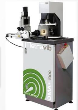
DMA testing device
