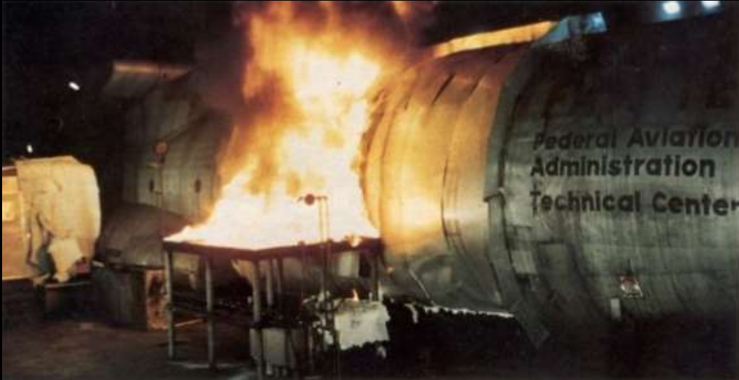
Post-crash fire simulation in full scale indoor at FAA
