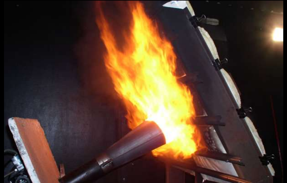
Burnthrough test (NexGen)
