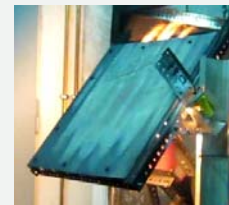
Carbon/geopolymer panel - Flame penetration test per FAA AC 20-135 (15 th minute)
