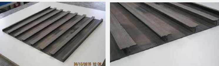
Carbon/geopolymer panel with „T“ integral stiffeners. Manufactured in single curing operation
