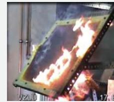
Glass/phenolic panel - Flame penetration test per FAA AC 20-135 (1 st minute)
