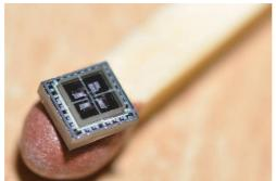
Figure 4-2: MEMS can vary in size from 1 to 100 microns, taken from [146]
