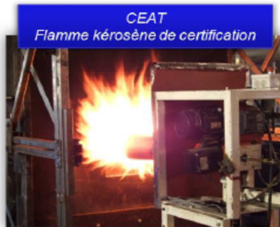
Figure 3 – Burnthrough test on an aircraft material panel
