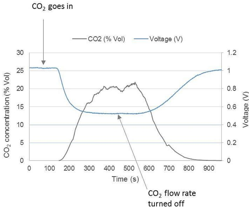
**Figure 8 Response of CO<sub>2</sub> sensor to a standard concentration of 20% CO<sub>2</sub> at a flow rate of 1 litre / min.**
