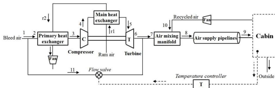
**Figure 1 Schematic of typical ECS system in aircraft. (C) corresponds to compressor, turbine (T), r (ram air), taken from [9]**
