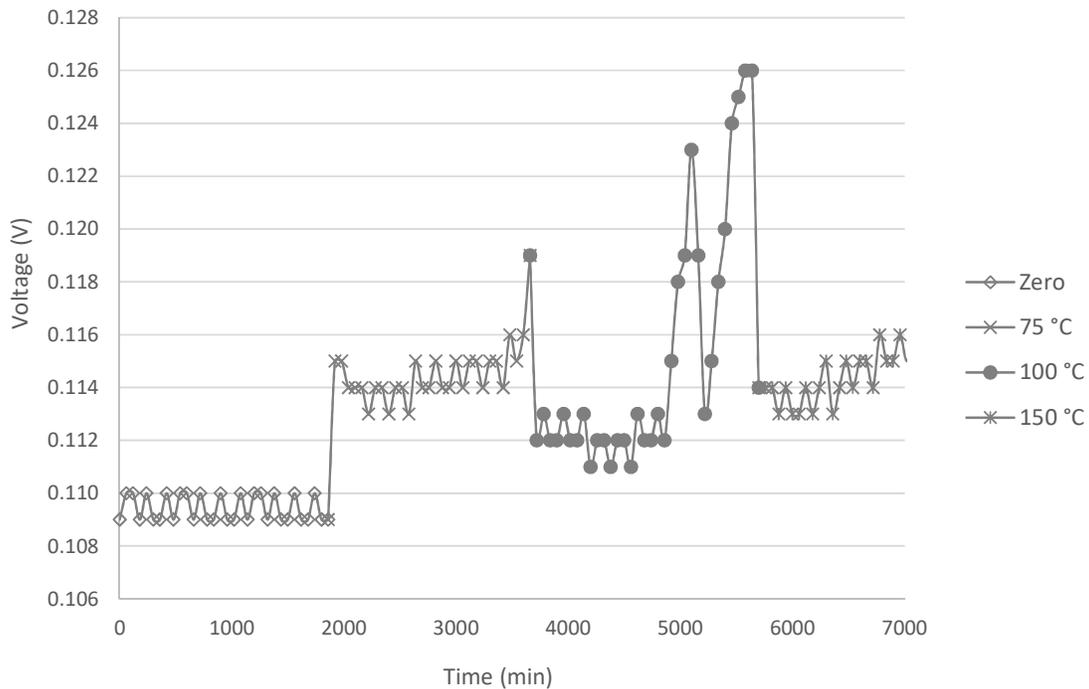
**Figure 9 Example response of the PID sensor to volatile emissions (furnace temperature controller programmed to warm up from 22 °C to 150 °C at 5 °C min<sup>-1</sup>).**
