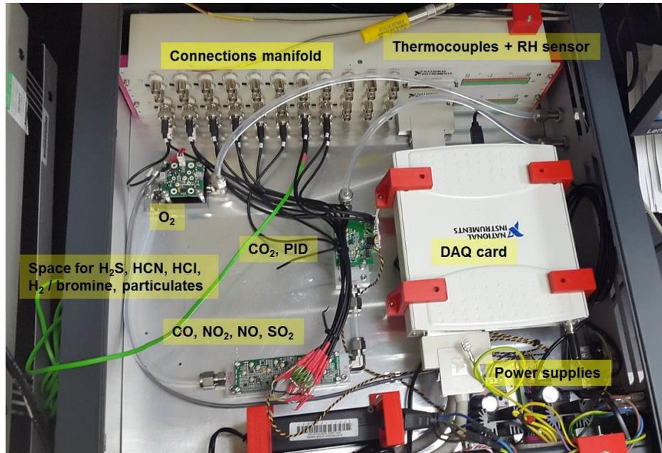
**Figure 7 Sensors box equipped with COTS gas sensors. Labels are highlighted in yellow.**
