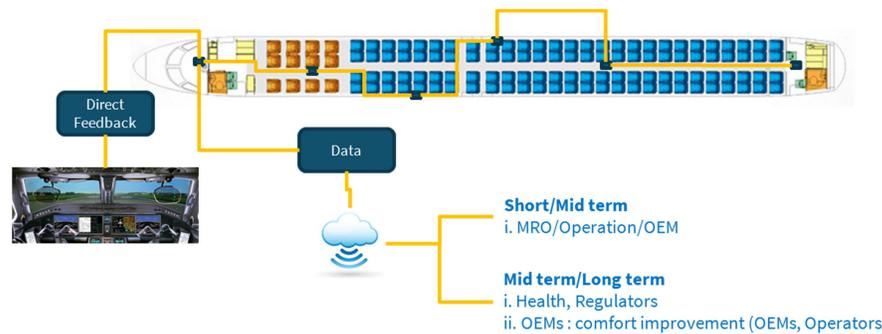
**Figure 10 Concept architecture for an Industrial cabin air quality Framework based on Continuous Air quality Sensing (IFCAS) (with cabin and cockpit pictures from Embraer)**
