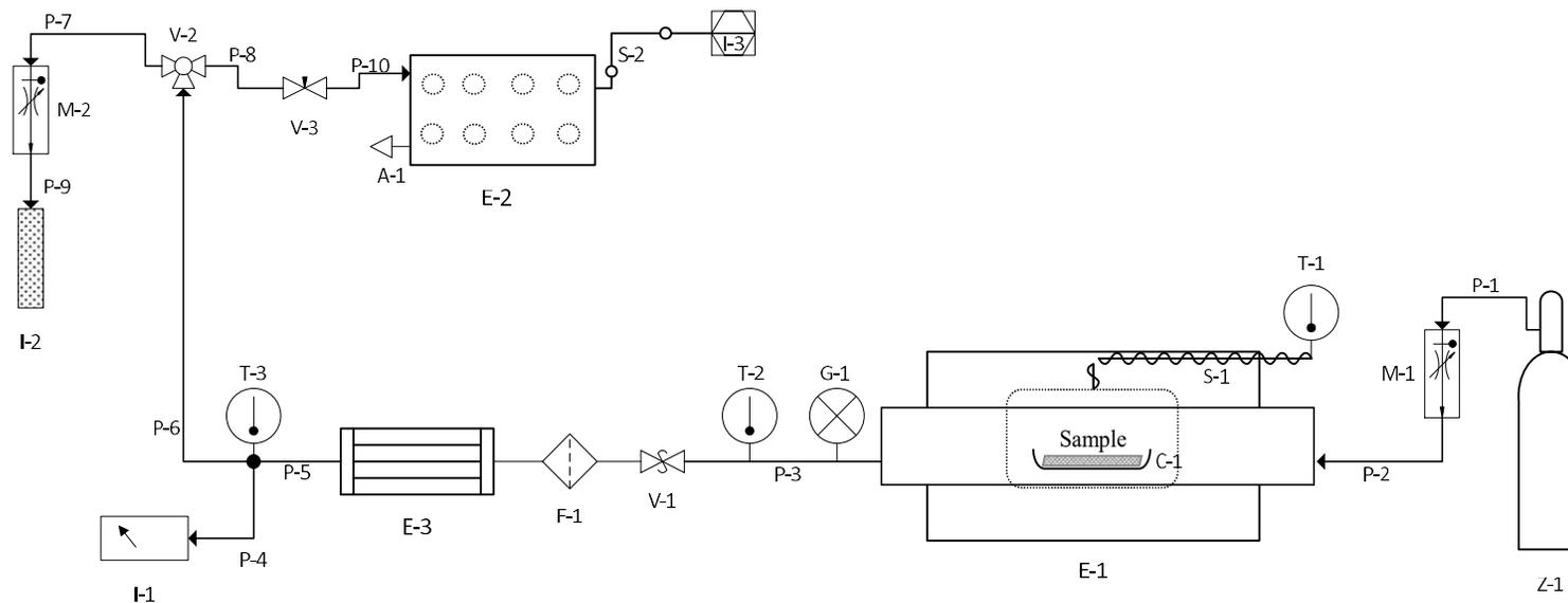
**Figure 5 A schematic diagram of the methodology for characterisation of gas emissions at elevated temperatures in real-time using commercial gas sensors and thermal desorption tubes.**
