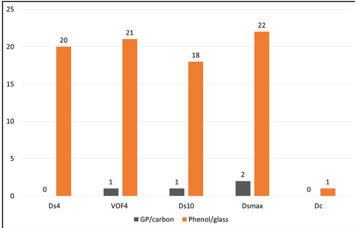
Figure 8: Smoke optical density
