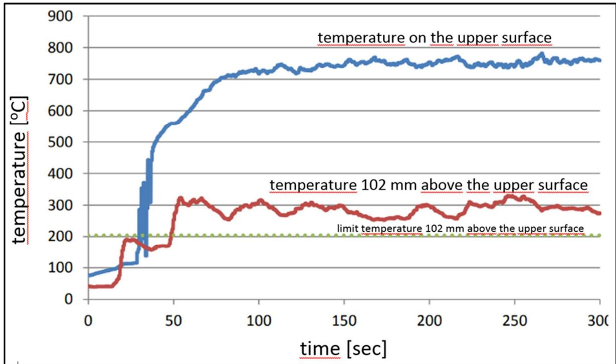
Figure 18: Referential glass/phenolic panel (honeycomb core): flame penetration test temperature record
