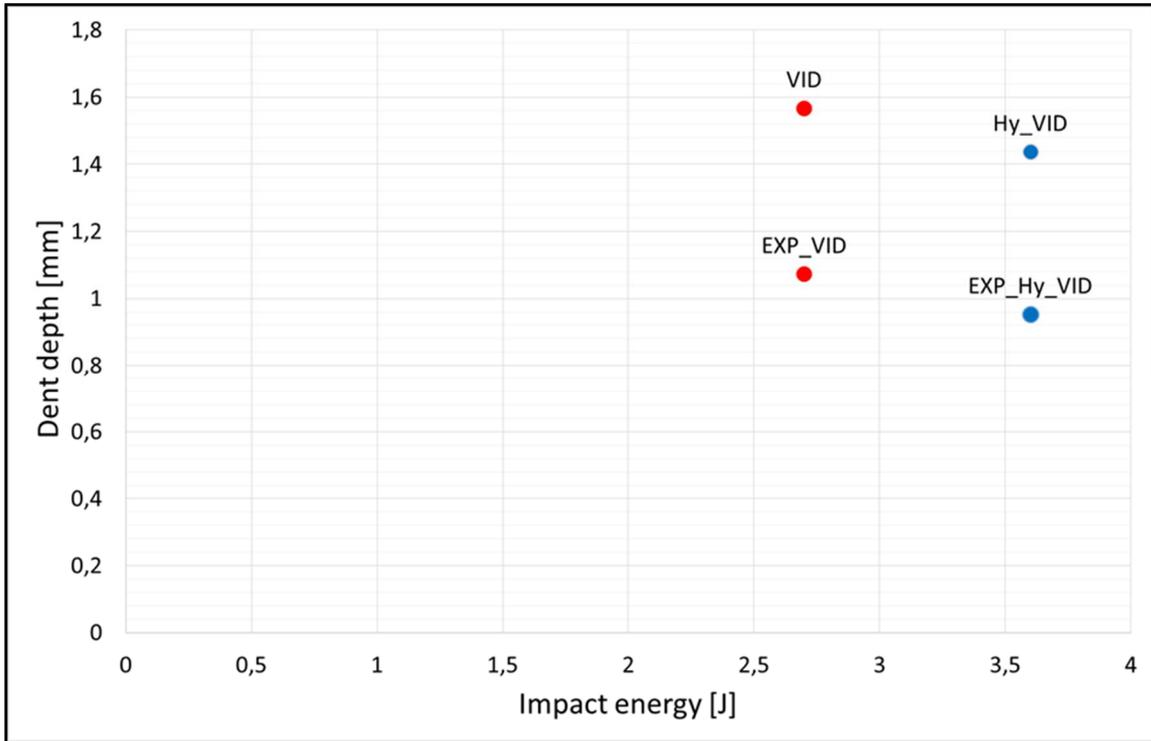
Figure 24: VID hot/wet exposed („EXP“) specimens showed approx. 30% better impact resistance compared to non-exposed ones
