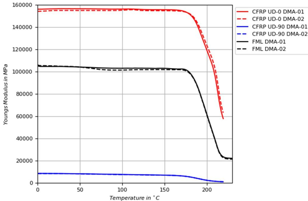
Figure 46: DMA results of FML and its cfrp components
