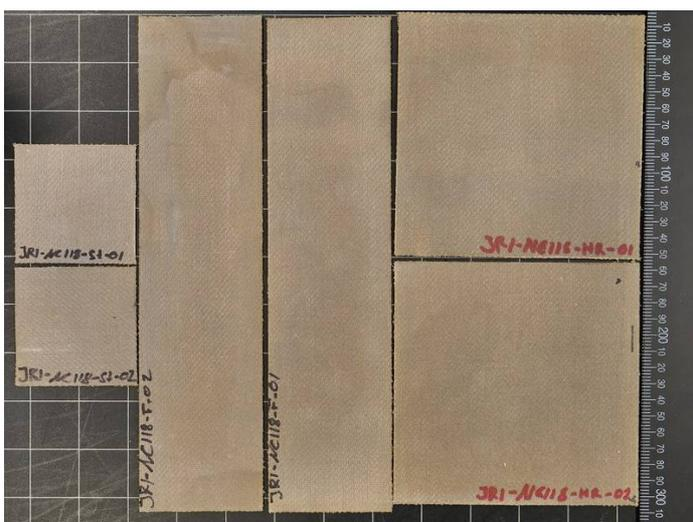
**Figure 34: Samples for the F, ST and HR tests made of flax plain fabric and Geopolymer matrix**
