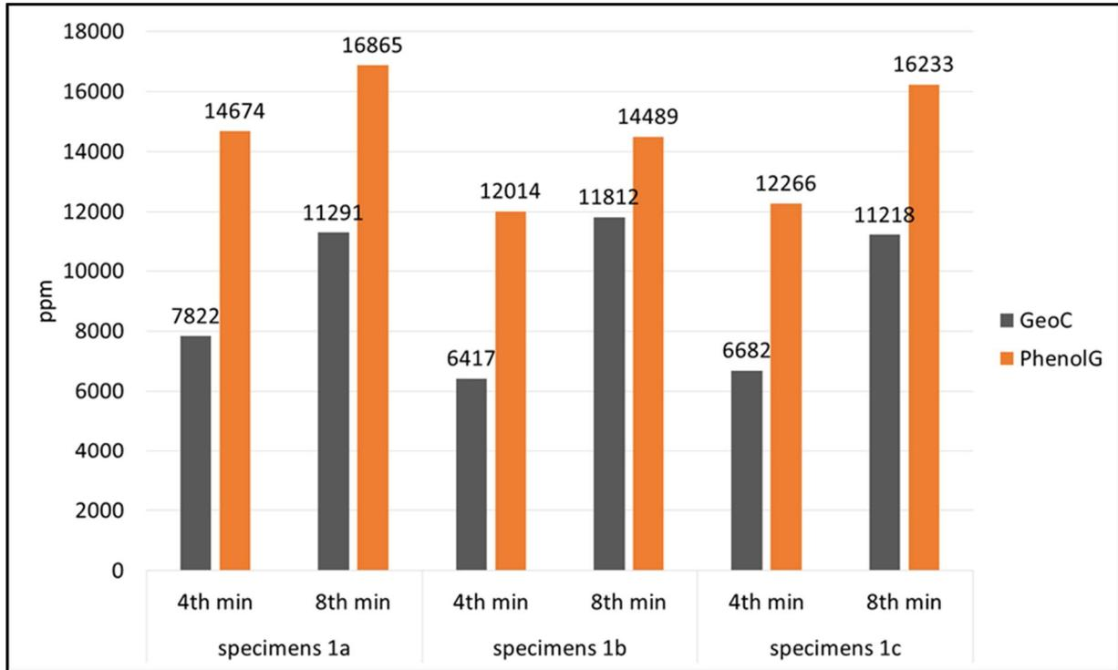
Figure 6: CO2 concentrations under test conditions
