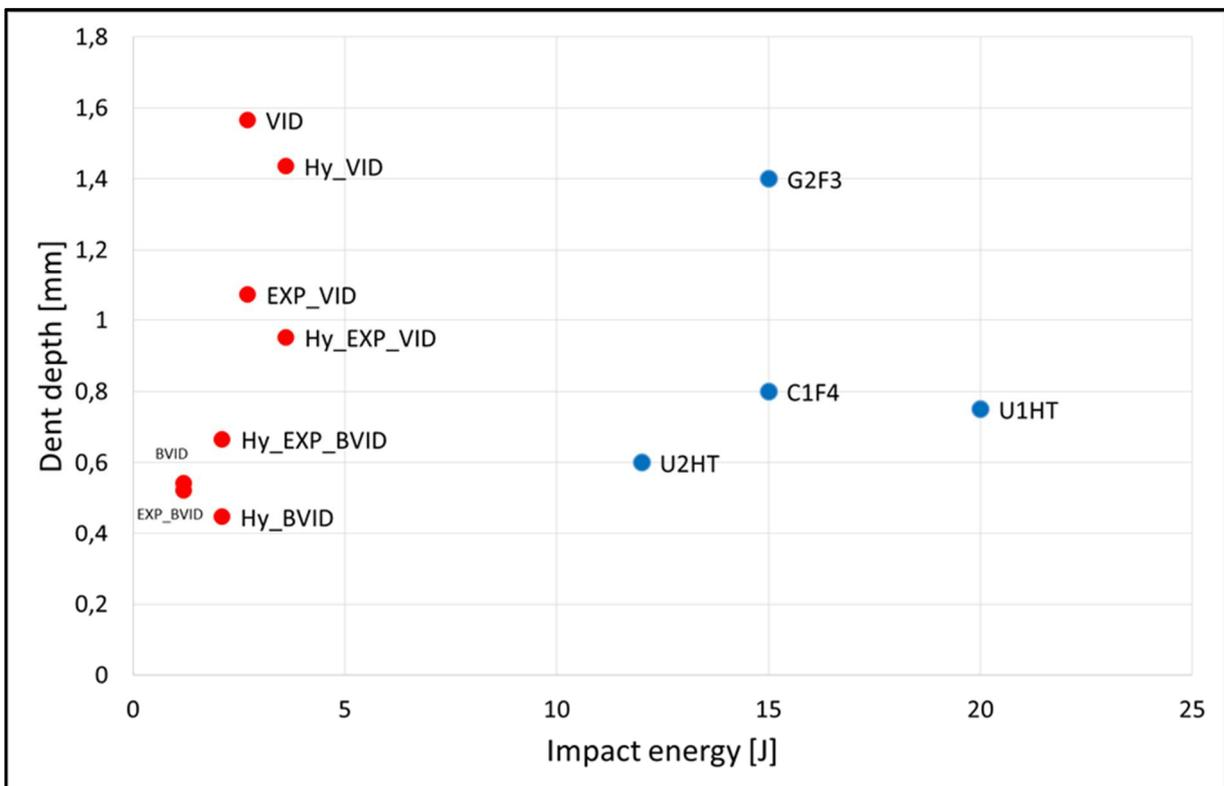
Figure 25: Comparison of impact resistance of Type 1 and Type 2 (red dots) specimens and referential specimens made of carbon/epoxy (blue dots)
