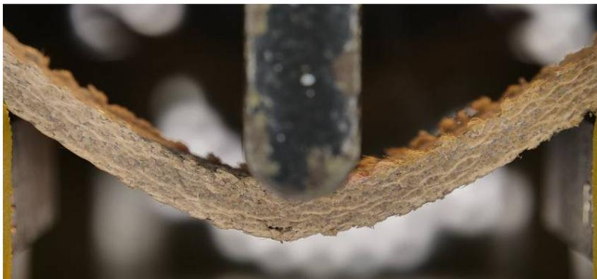
**Figure 40: Considerable deflection of flax fabric + GPL sample during flexural testing**
