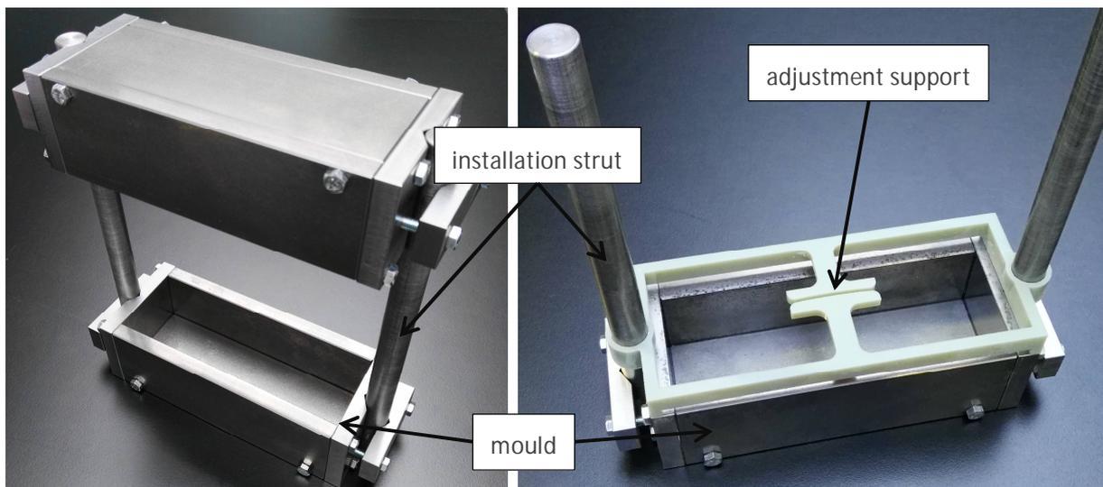
Figure 44: Specimen device; Installation struts and adjustment support are removed after moulding of the specimen
