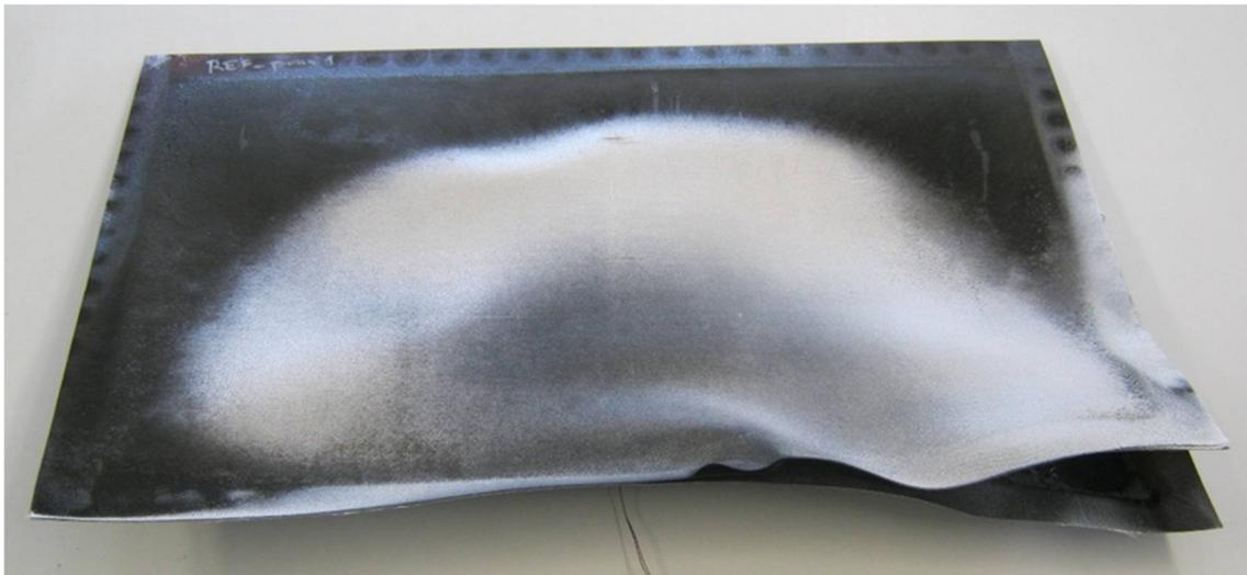
**Figure 13: Exposed side of the referential glass/phenolic panel after the test. White spot is a glass fabric where phenolic resin was completely burned off. Typical rupture can be seen on the edge of the panel**
