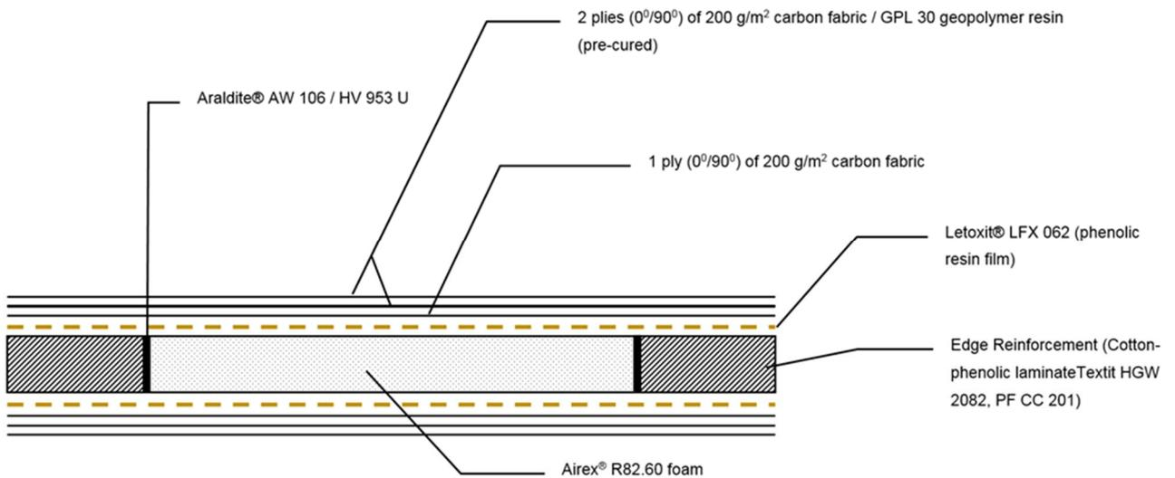
Figure 21: Lay-up arrangement of test specimens Type 2 (carbon/geopolymer/phenol hybrid)
