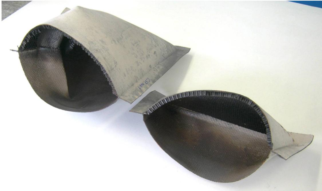
Figure 16: Split carbon/geopolymer panel after the test. No fire penetration or ruptures were registered.
