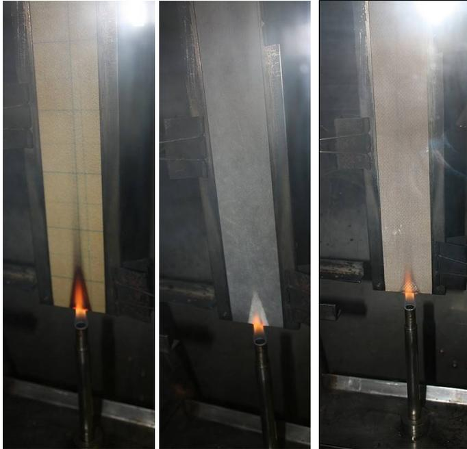
Figure 35: During the Flammability test (12s, vertical): GF+PF reference (left), rCF+GPL (middle) and flax+GPL (right).
