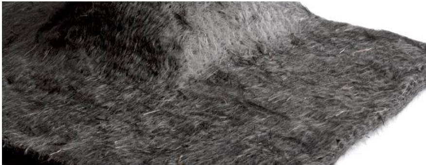
Figure 2: rCF nonwoven “Carbiso M” by ELG Carbon Fibre Ltd. [ELG Carbiso M data-sheet, available online at: <http://www.elgcf.com/assets/datasheets/Carbiso-M.pdf>]
