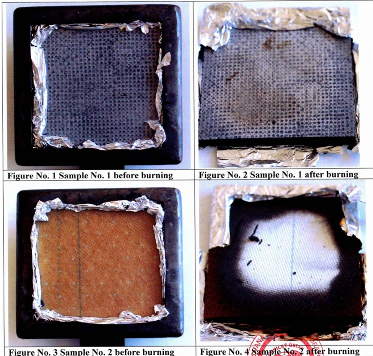
Figure 10: Materials samples before and after burning. Carbon / geopolymers above (Fig. No. 1, Fig. No. 2), glass / phenol below (Fig. No. 3, Fig. No. 4). White spot surrounded by soot on Figure No. 4 is a glass fabric where phenolic resin was completely burned off
