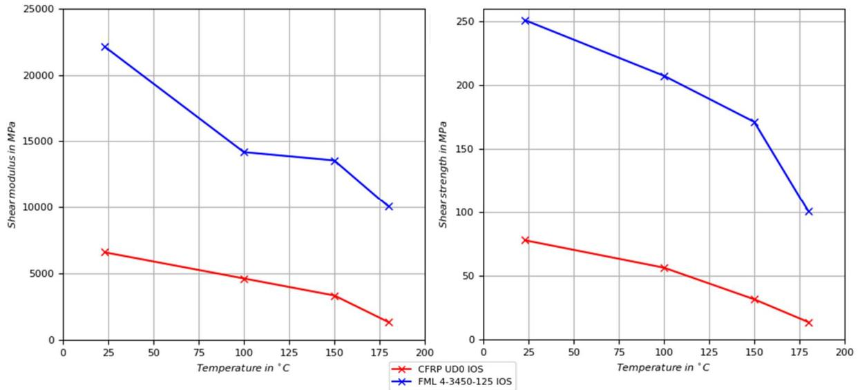
**Figure 47: Temperature dependent shear properties of FML and cfrp from test results according to ASTM D 5379**
