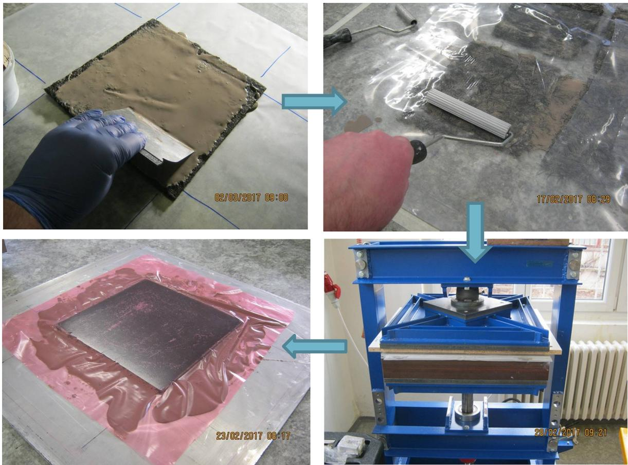
**Figure 30: Manufacturing of composites with Geopolymer matrix (VZLU)**
