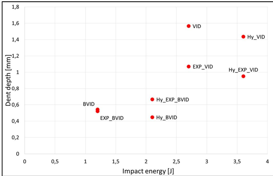
Figure 23: Functionality of impacts depth on impact energy for Type 1 and Type 2 („Hy“) skins
