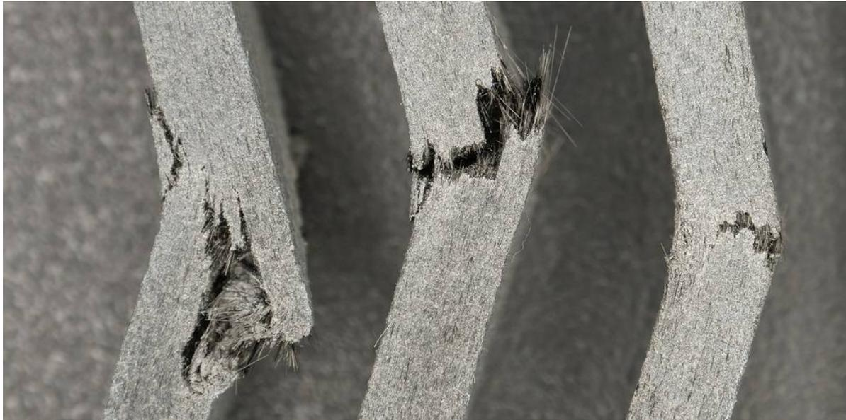
**Figure 42: Fracture of rCF+GPL sample after flexural test (side view)**
