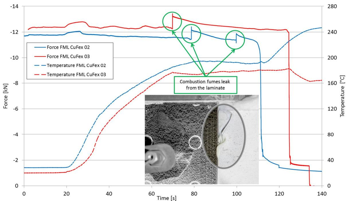
**Figure 45: Force and temperature curves of two exemplary CuFEx-specimens**
