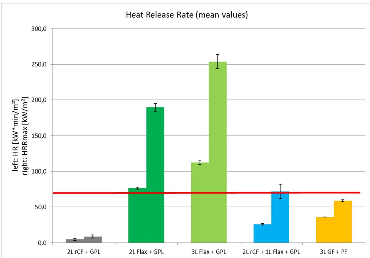
**Figure 37: OSU results for Heat Release (left column for each material combination) and Heat Release Rate (right column) of the eco-fibres with GPL matrix and GF-PF reference according to FAR 25.853. The red line indicated the limit of 65 kW/m<sup>2</sup> respectively 65 kW\*min/m<sup>2</sup>.**
