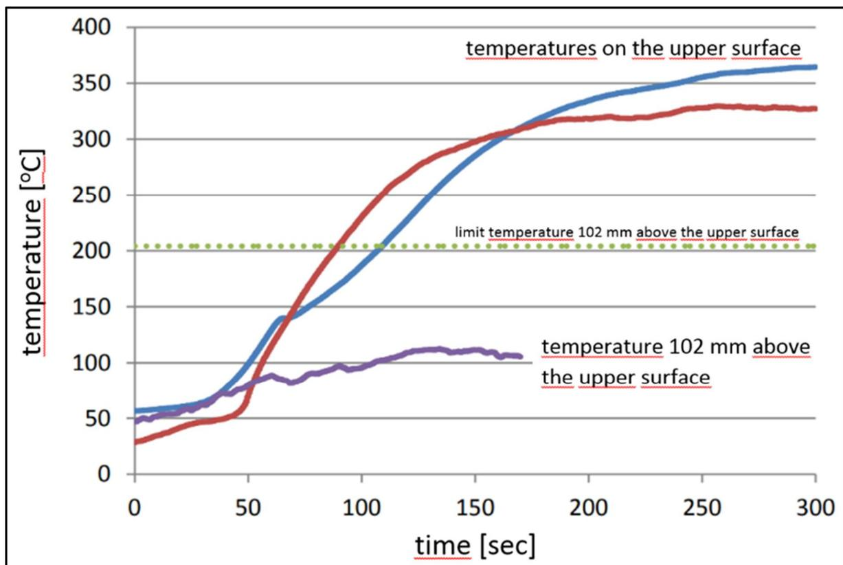
Figure 17: Carbon/geopolymer panel (honeycomb core): flame penetration test temperature record
