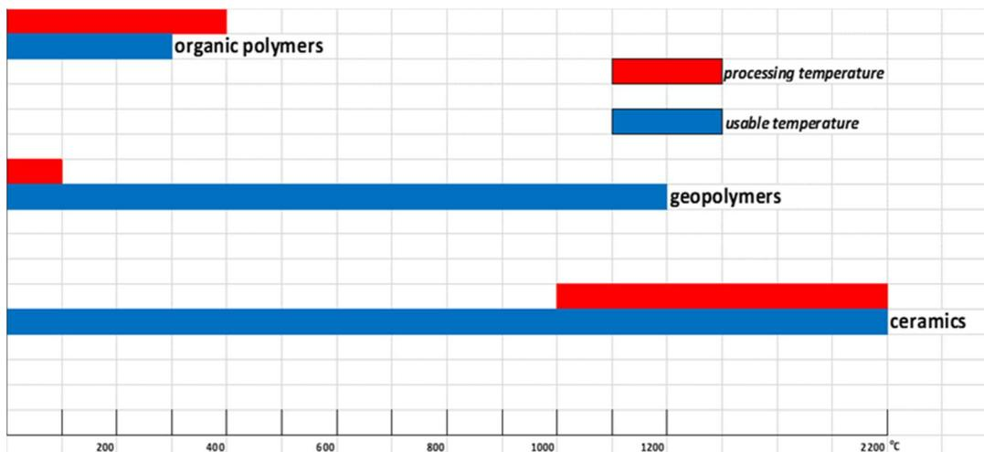
**Figure 1: Processing and usable temperatures „windows“ of composite matrixes**
