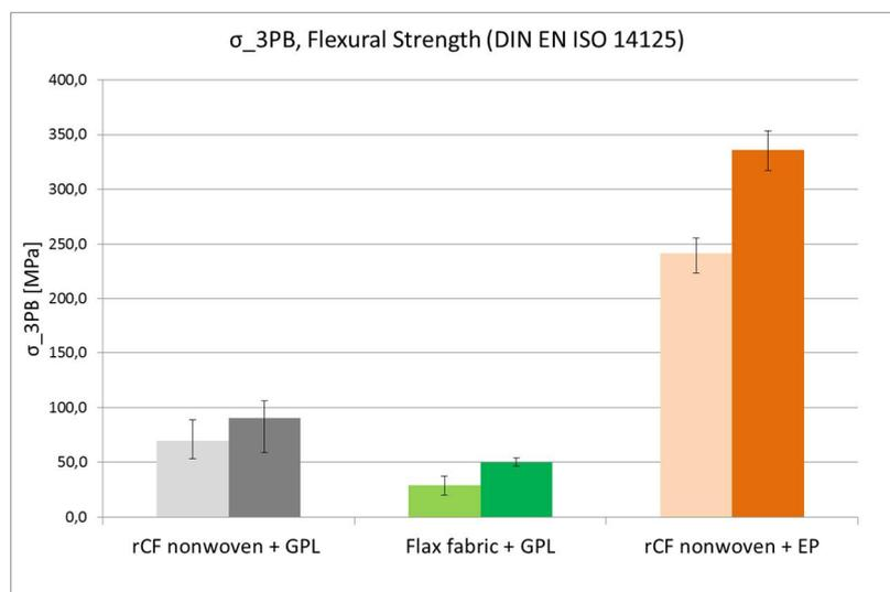
**Figure 38: Flexural Strength**
