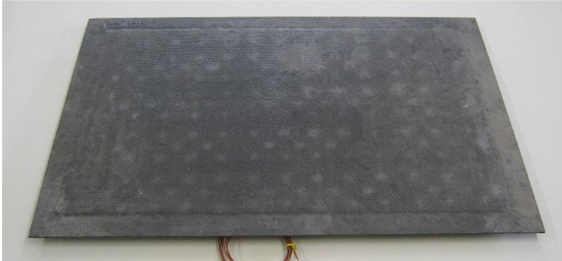
**Figure 14: Exposed side of carbon/geopolymer panel before the test**
