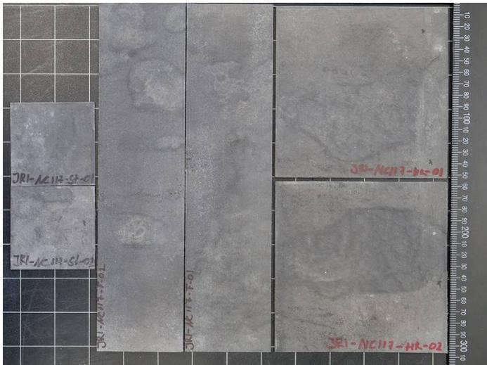
**Figure 33: Samples for the F, ST and HR tests made of rCF nonwoven and Geopolymer matrix**
