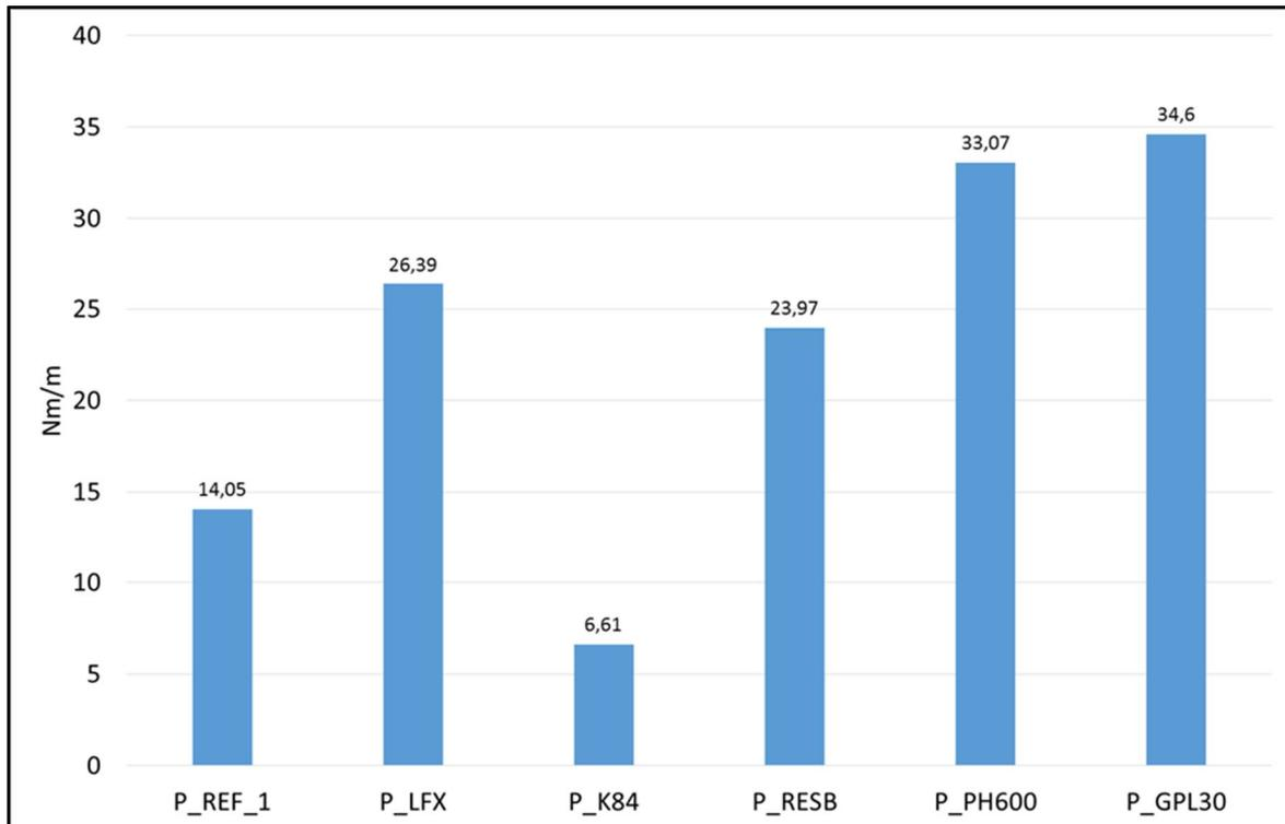
Figure 26: Average peel strengths of foam core specimens
