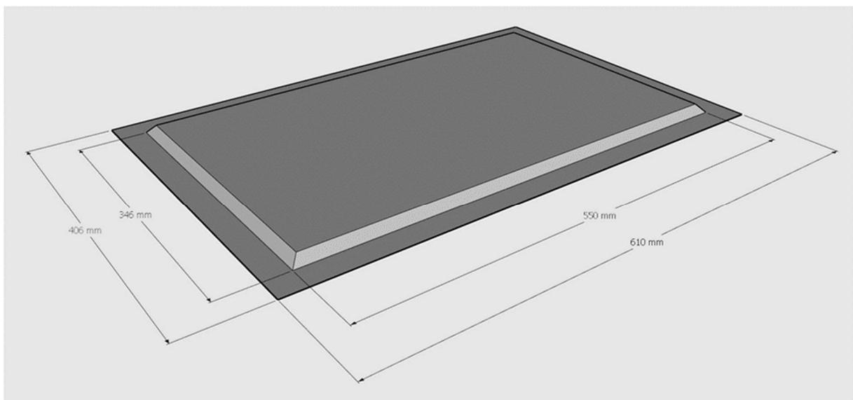
**Figure 11: Sandwich test panel – geometrical scheme (core thickness 10 mm, core edges 45° chamfered)**
