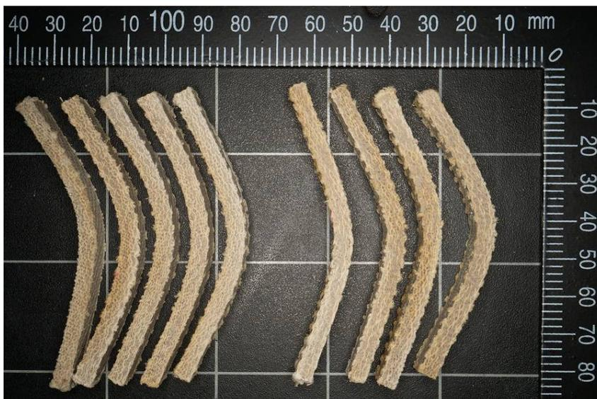
**Figure 41: Samples after testing (flax fabric + GPL, left = 0°, right = 90° test direction)**
