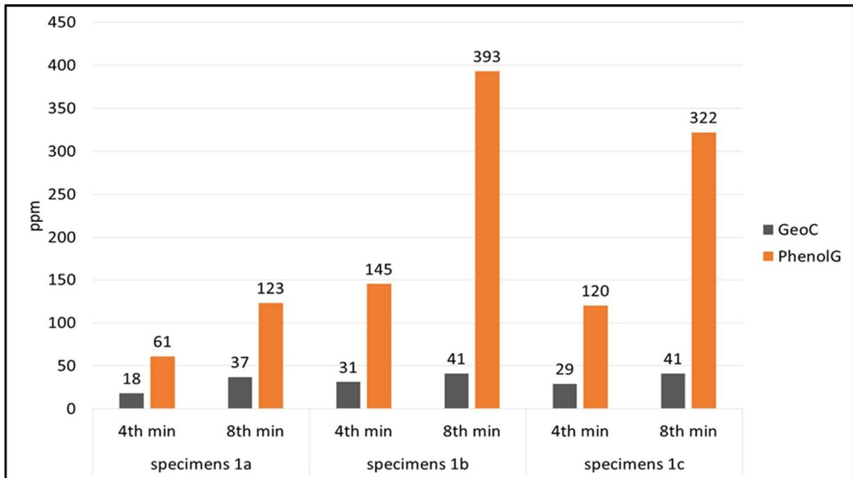
Figure 5: CO concentrations converted to standard pressure and temperature (101.325 kPa, 25°C)
