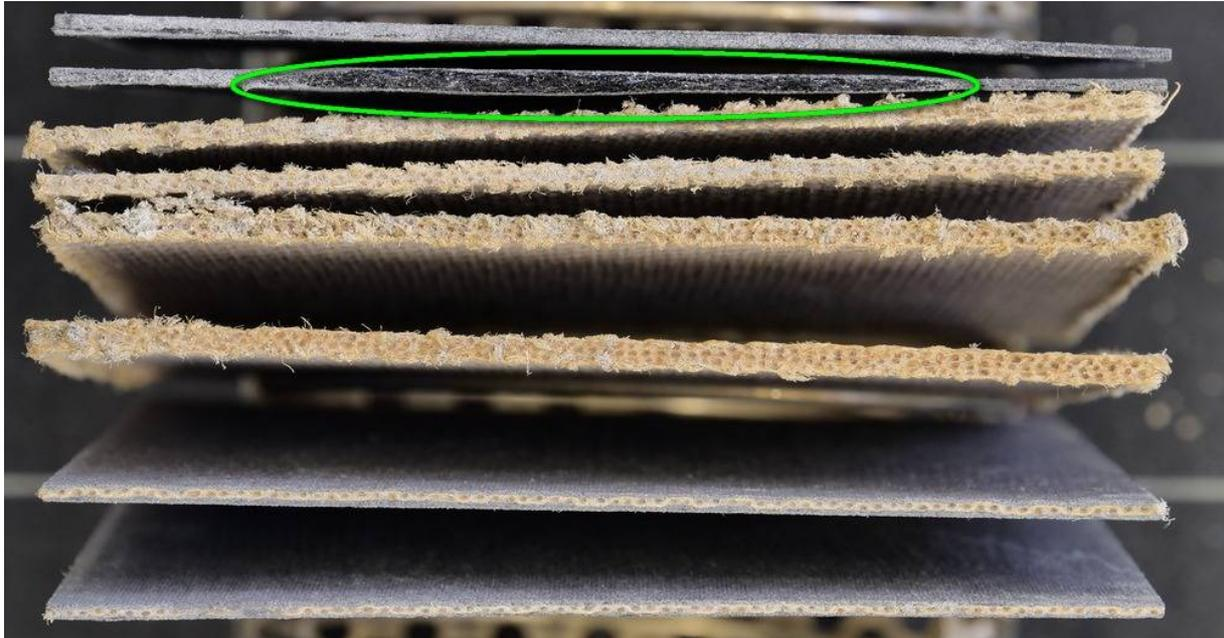
Figure 31: Dry area visible in the centre of a smoke density test specimen reinforced with 2 layers of rCF nonwoven and Geopolymer matrix (specimen side length 73mm, thickness approximately 1mm)
