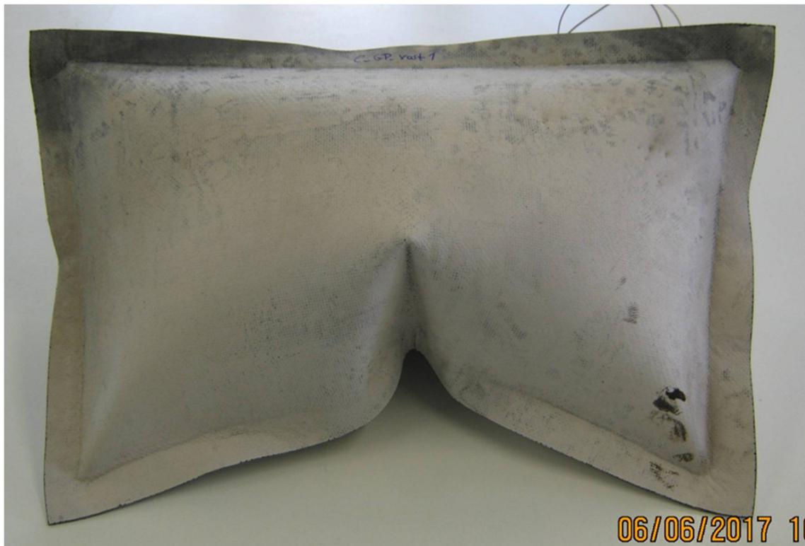
**Figure 15: Exposed side of carbon/geopolymer panel after the test. Typical "pillow effect" is evident**
