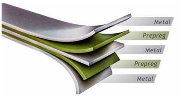
Figure 3: Lay-up of fibre metal laminates (schema) [<http://unitedglassply.com>]
