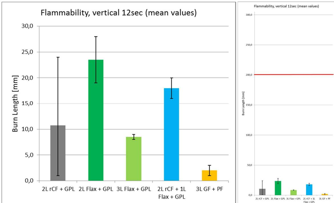
Figure 36: Flammability of the eco-fibres with GPL matrix and GF-PF reference according to FAR 25.853. The right hand figure shows the same results in relation to the specimen length. All results are far below the limit burn length of 203mm indicated by the red line.
