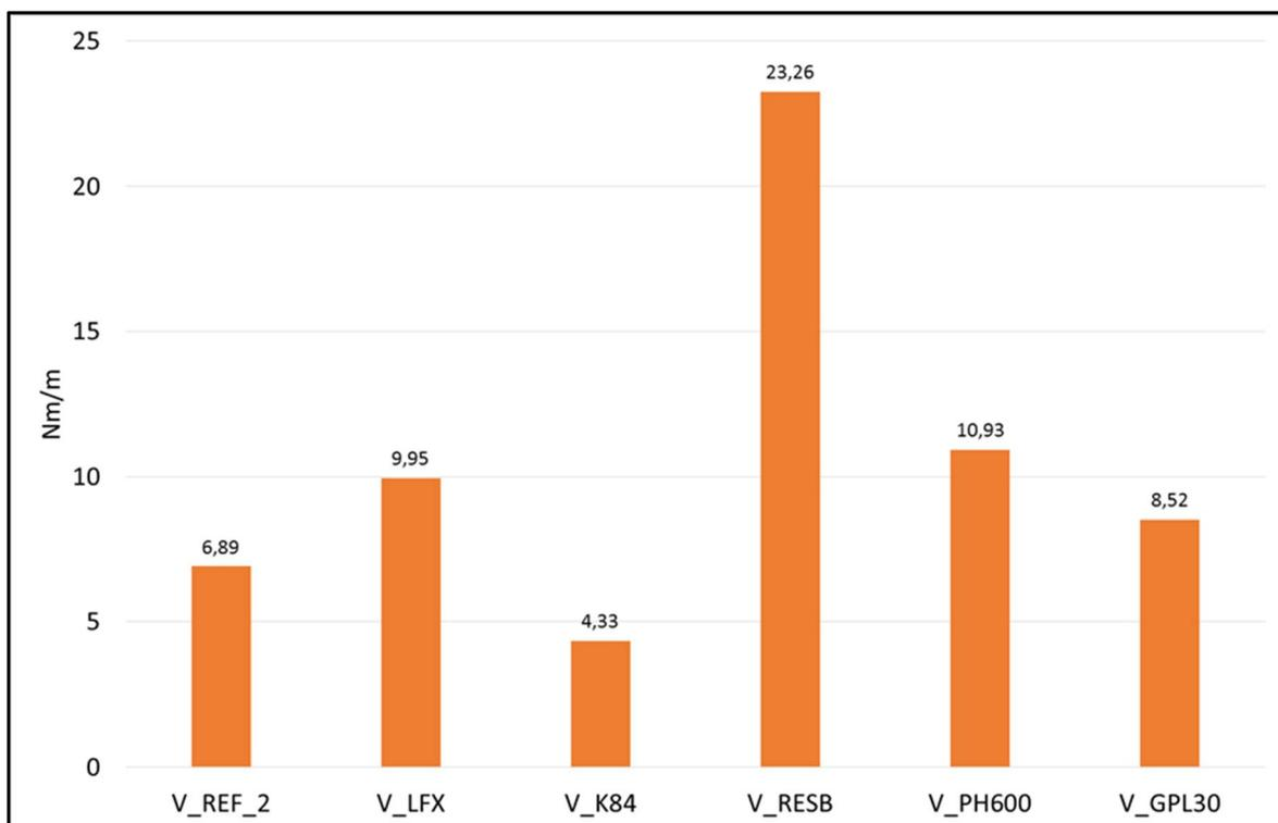
Figure 27: Average peel strengths of honeycomb core specimens
