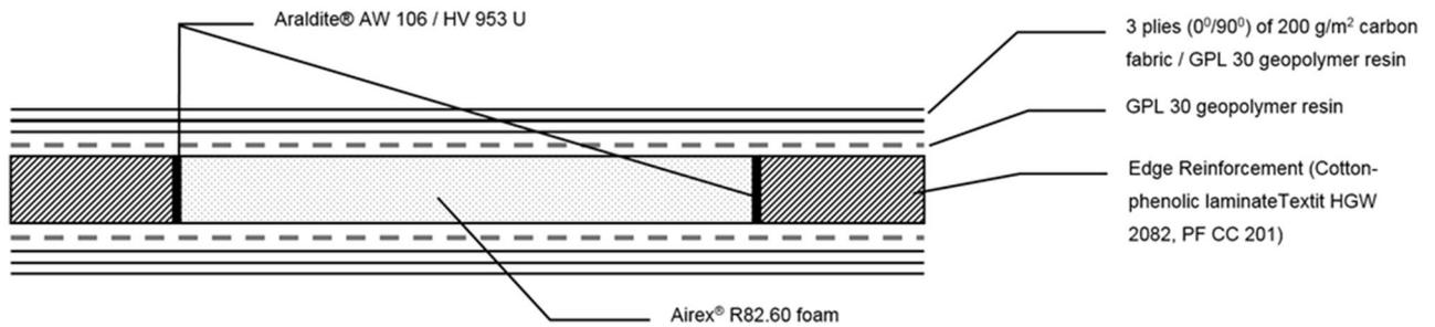
Figure 20: Lay-up arrangement of test specimens Type 1 (carbon/geopolymer)
