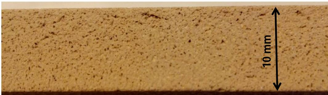
**Figure 29: Detail of the geopolymer foam structure**
