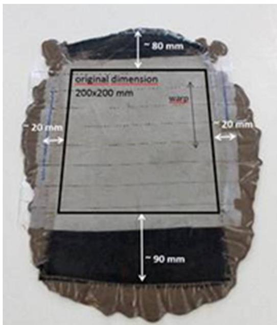
Figure 32: Expanded surface area (mainly in nonwoven machine direction (MD)) observed during the production of rCF nonwoven reinforced Geopolymer (20 layers) in a hydraulic press
