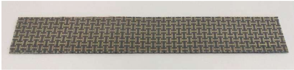
Figure 42: Test specimen for the vertical test made of carbon-aramid-geopolymer hybrid composite (50 x 305 mm , mean thickness 1,05 mm, specific weight 1,45 g/cm 3 )
