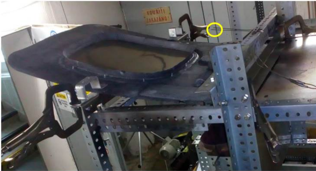
Figure 32: Flame penetration test: two thermocouples (in yellow circle) located 100 mm above the back surface
