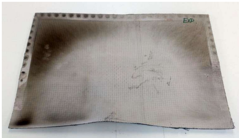
Figure 39: Exposed side after the test
