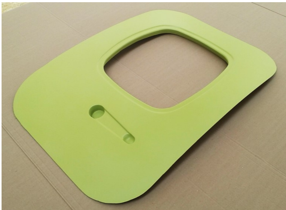
Figure 27: Outer side of the molding A (surface filled and painted)
