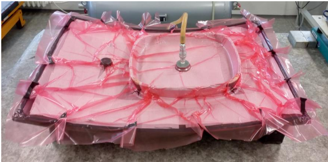
Figure 23: All plies of the Demonstrator were proceeded by wet-laminating method. Standard vacuum bagging process (-95 kPa, R.T., overnight curing) was typically applied
