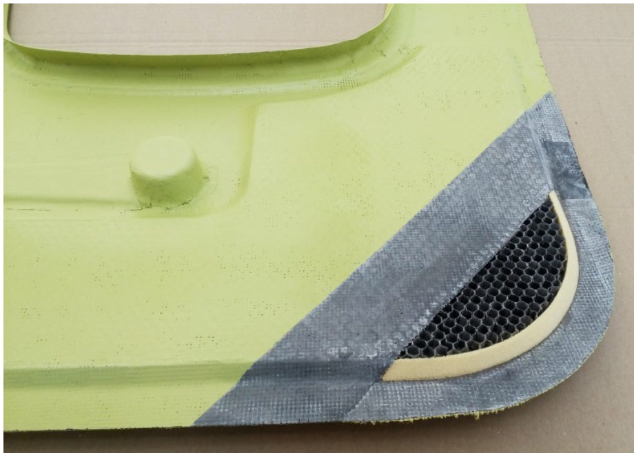
Figure 29: Detail of the sandwich core (molding A)
