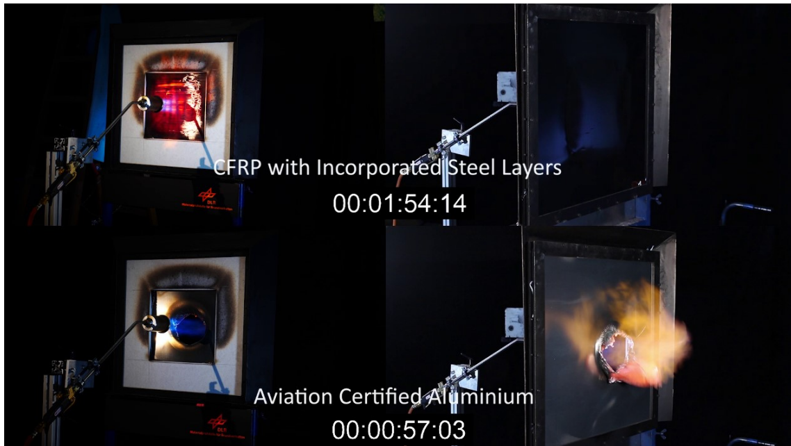
Figure 48: Comparison of the fire response of a FML test panel and an aluminium certified test panel submitted to a flame penetration test
