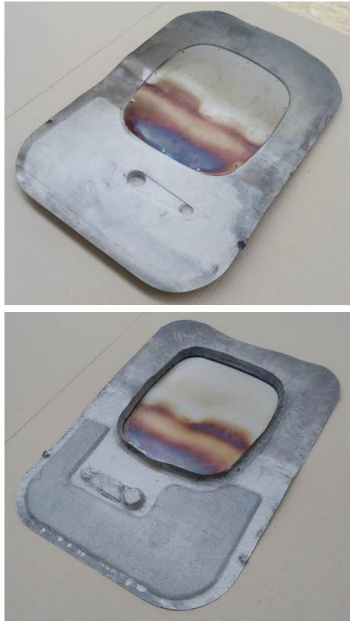
Figure 34: Molding B after 10 minutes of the flame penetration test. Exposed side (above) and back side (below). After the test, no visible changes have been registered on the molding, except of colour change and warpage of the edges. Due to application of geopolymer honeycomb, no sandwich “pillow effect” was registered. The molding has maintained integrity and very good stiffness
