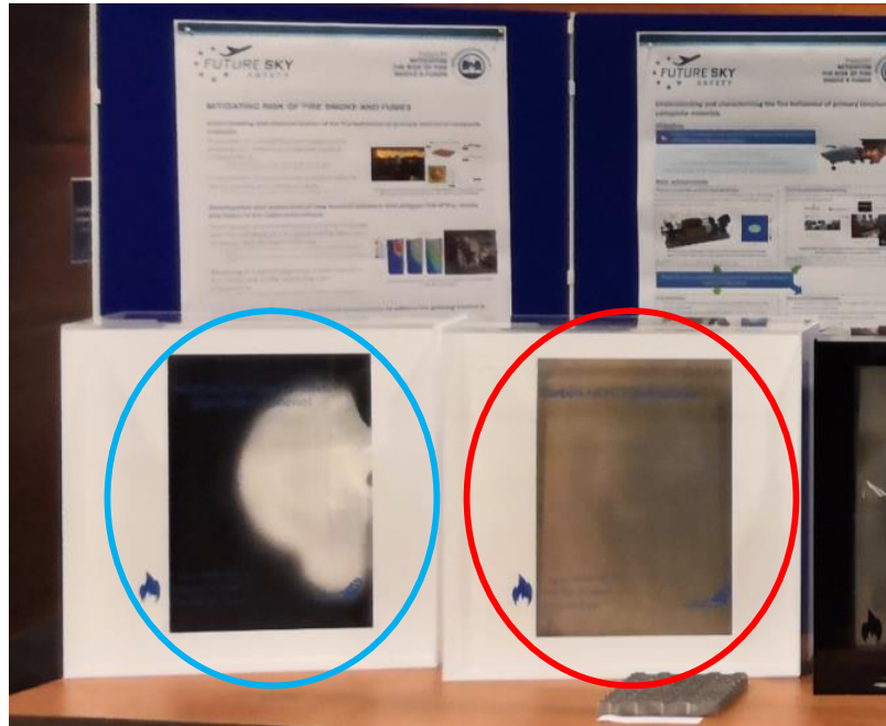
Figure 5: Demonstrator No.1 (right) and referential glass/phenolic panel (left), both after the flame penetration test, as they were presented on FUTURE SKY SAFETY Final Conference (November 2018, Eurocontrol Headquarters, Brussels)
