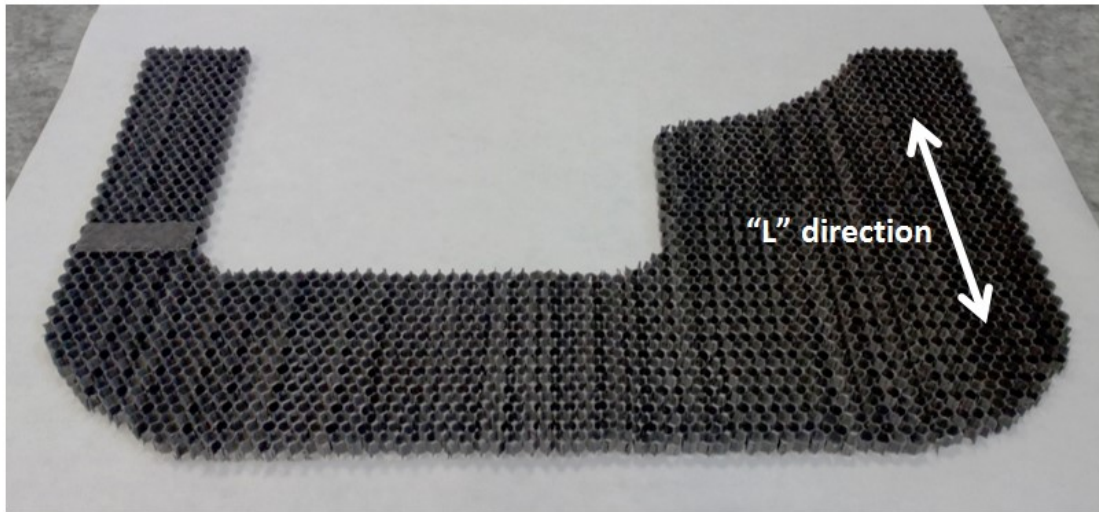
Figure 21: The sandwich core. Specific weight of the honeycomb is approx. 234 kg/m 3
