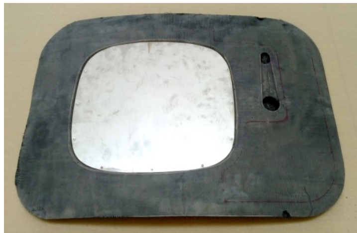
Figure 31: Molding B prior to the flame penetration test. Window cutout was covered by 0,5 mm stainless steel
