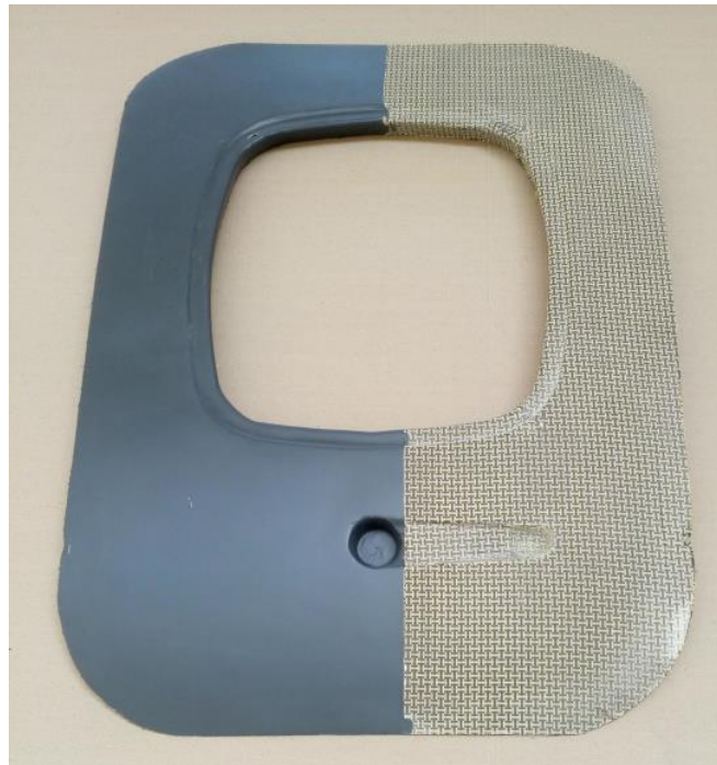
Figure 37: Molding C (primer paint applied on the left half)
