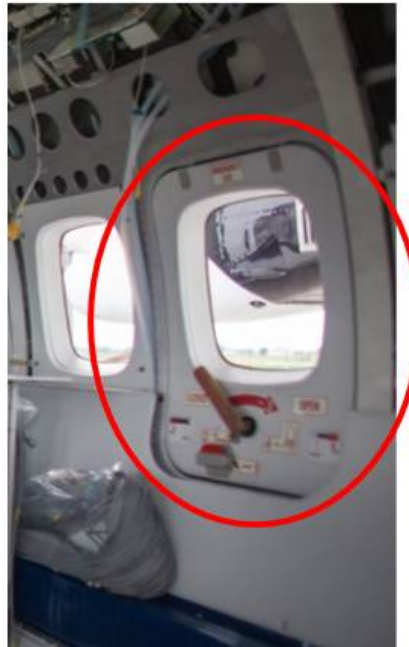
Figure 6: Emergency exit door [www.aktualne.cz]
