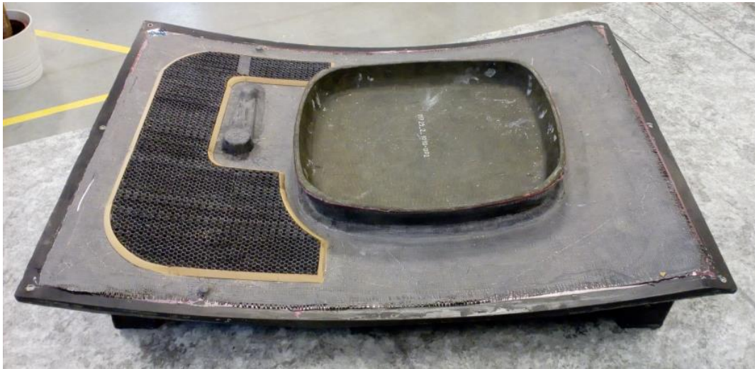
Figure 24: Honeycomb core (dwg. positions 010, 005) assembled and bonded on cured outer skin
