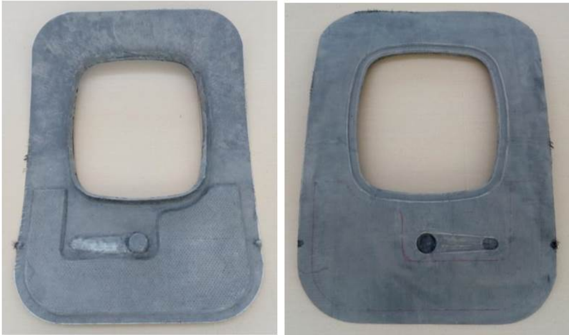
Figure 30: “Bag side” and “tool side” of the molding B
