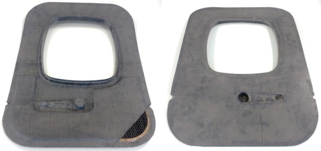
Figure 26: “Bag side” and “tool side” of the molding A prior to painting. Weight of trimmed molding A (without surface finish) was 770 g
