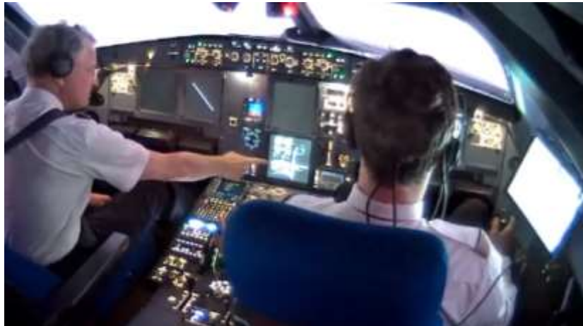
Figure 73: State of the display panels during the AC bus failure
