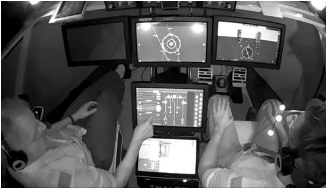
Figure 75: Crew engaged in the ECAM action procedure with the Thales new avionic interfaces. During the AC bus failure, the captain PFD is no longer available and the ECAM actions are managed thanks to the central system display
